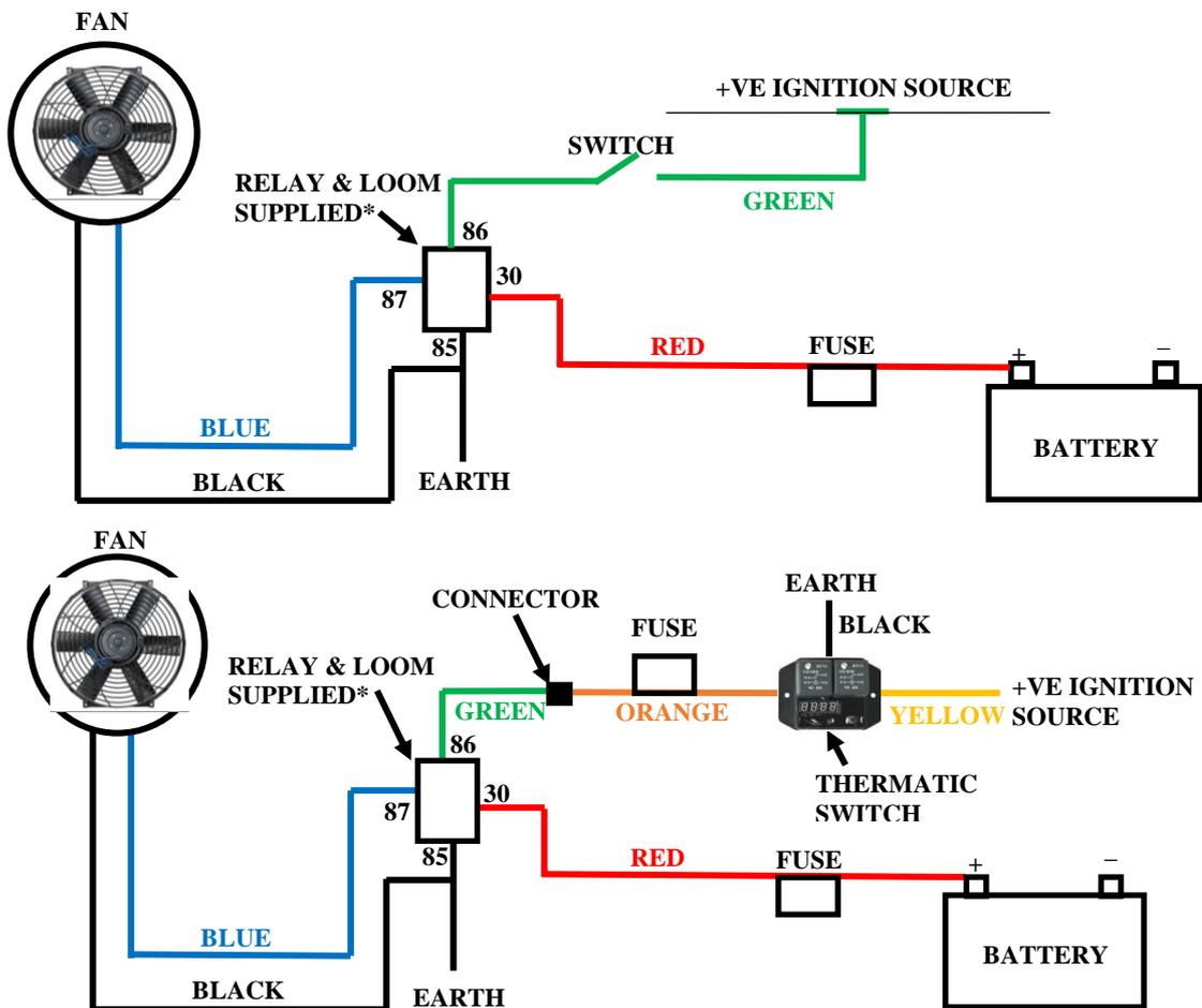
**Figure 6** –Wiring Diagram for Standard Set-up **a.)** without Thematic Switch or **b.)** with Thematic Switch (Part #0444). \* **Note:** Relay, Loom, Connector & Fuse are supplied with Part #698 and #691 only.
