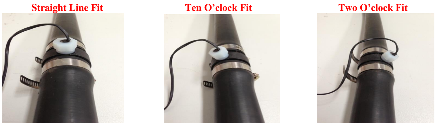
Fig.3 – Inline Sensor Adaptor Fitting Positions
