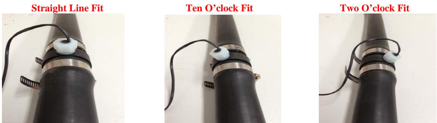
**Fig.3 – Inline Sensor Adaptor Fitting Positions**
