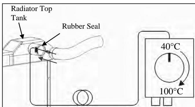
Fit the hose and clamp so that the clamp is over the centre of the rubber seal and the clamp screw is in the opposite side of the tube to the capillary and seal. *A good silastic type sealant may be useful if there is a persistent leak.*
