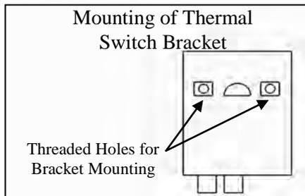
3. Mount the bracket onto a panel near the radiator so that the stainless steel bulb will easily reach into the top radiator hose. Ensure that the adjustment shaft is accessible. Fix the bracket in place with the two large self-tapping screws provided.
