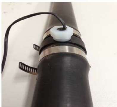
Fig.3 – Inline Sensor Adaptor Fitting Positions
