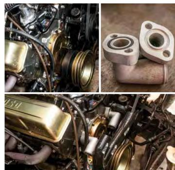
To fit the kit with the header kit, which is essentially two short elbows that bolt to the stock water pump bolt holes and a specific piece of hosing, first we removed the stock pump.
