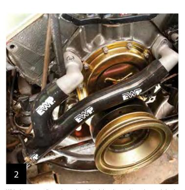
With the two top lines trimmed, we fitted the pipe to the outlets and sized up the lower piece with the EWP, making sure it was suspended in mid-air and not fouling on the chassis rail. Once happy, we secured it with the provided T-bolt clamps.
