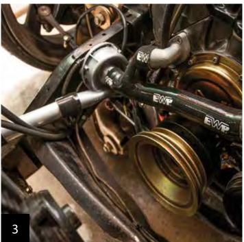
To link the pump and lower radiator inlet, there are a few options. You can use a silicone hose, chop down the factory radiator hose to length, or, like us, use a short length of alloy pipe with the silicone offcuts as joiners. There is no real advantage of one way over another.
